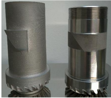
Figure1 - As built vs superficial polished Inconel part
