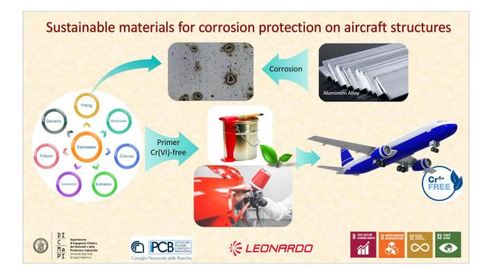
In recent years, chromates, widely used as anti-corrosion pigments in primers and wash primers, have completely disappeared in most industries due to the detrimental effects of hexavalent chromium on the human health and the environment. However, many hexavalent chromium coatings are still used in the aircraft industry since the use of these coatings provides exceptional corrosion protection at relatively low cost.
