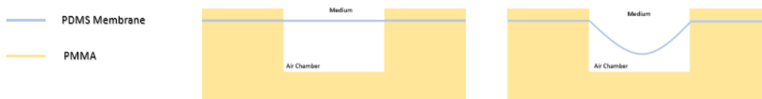
Figure 1 - Trasversal section of the microfluidic device
