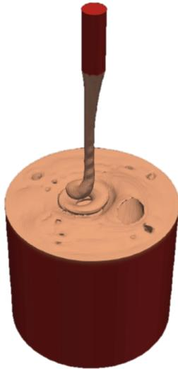
Figure 1 - CFD simulation of devolatilizer filling
